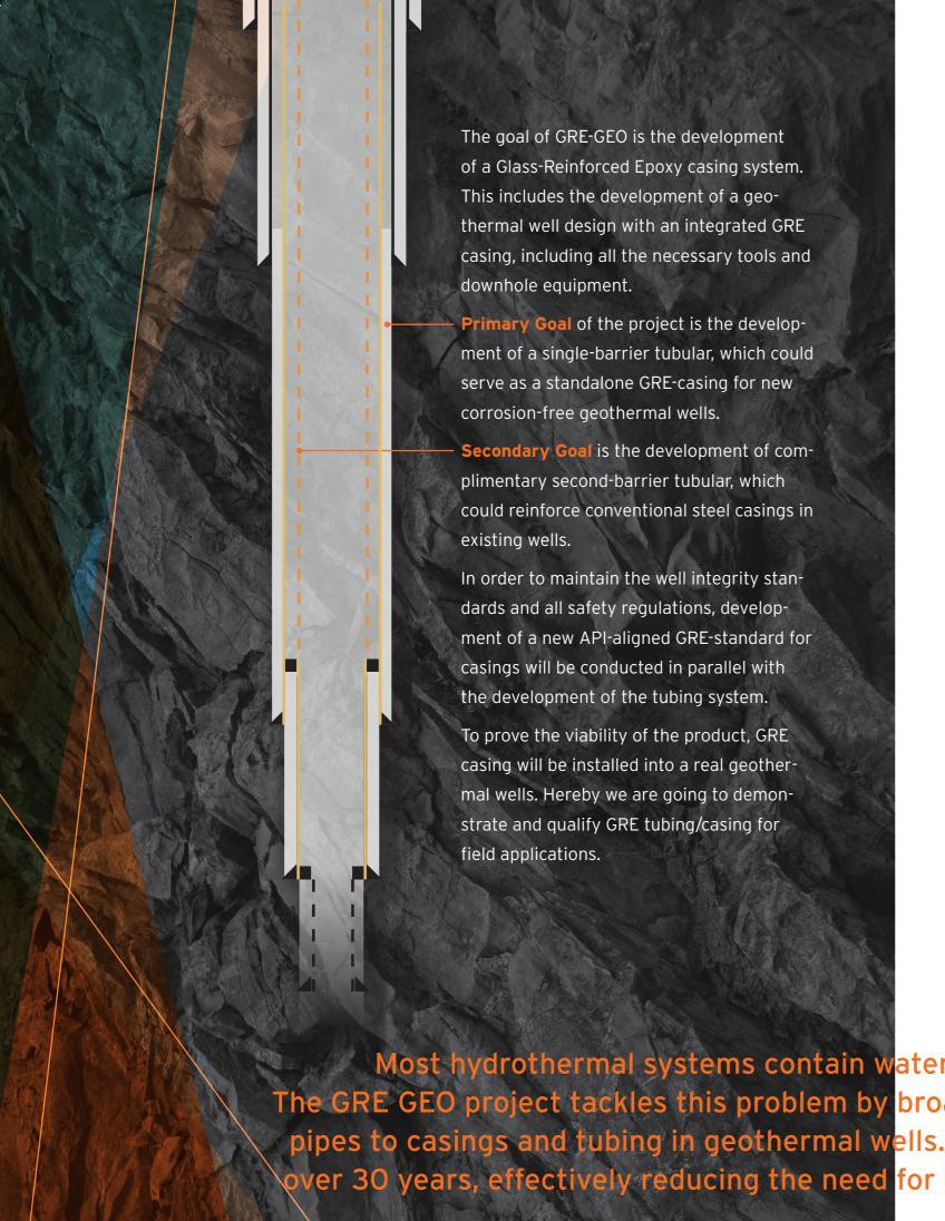
The success of the project implies development of a GRE pipe fit to utilization in subsurface conditions.
